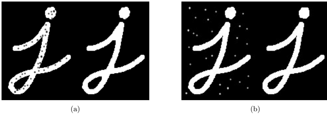
Figure 3.7: Complex morphological transformations [57]: (a) Closing; (b) Opening.
