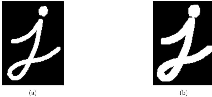
Figure 3.6: Dilated object with a (5 \times 5) rectangular kernel [57]: (a) Test image; (b) Dilated image.
