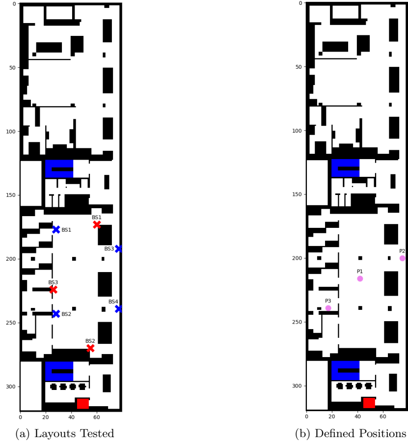
Figure 5.3: Layouts Tested and Positions Defined: (a) Layouts Tested - The red crosses are the BSs positions used for Layout 1, the blue crosses are the BSs positions used for Layout 2, each BS has its identification near it; (b) Defined Positions - The violet points are the defined positions for the measurements, each position has its identification near it.
