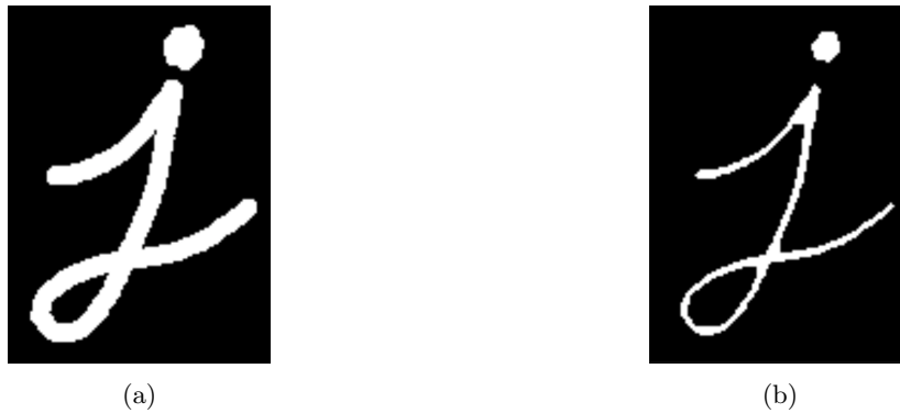
Figure 3.5: Eroded object with a (5 \times 5) rectangular kernel [57]: (a) Test image; (b) Eroded image.
