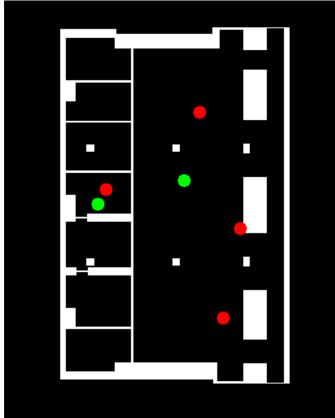
Figure 4.18: LOS Example. Assuming the pixels in red are BSs that can cover both points from the working area represented by the green pixels. In this scenario, both points would have coverage of four BSs, however, only the point in the middle would be considered to have LOS since it has no obstruction with at least three BSs.
